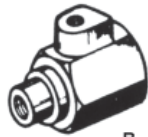
B. END CAP with residual check valve
