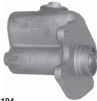
F42194 Ford applications Casting No.: FE41208 Ports: 1/2 X 20 G Bore: 1 1/2"
